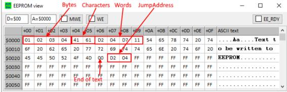
After assembling and programming the .eep file to the controller, its EEPROM looks like shown in the picture.
