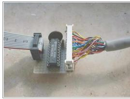
The necessary program algorithm is done by the ISP software. Be aware that this parallel port interface is not supported by ATMEL's studio software any more. So, if you want to program your AVR directly from within the studio, use different programmers. The Internet provides several solutions.
