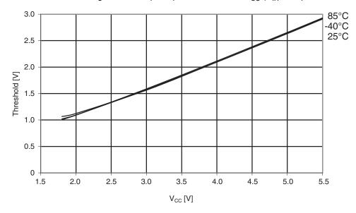
Figure 29-221. Atmel ATmega644A: I/O pin input threshold vs.  $V_{CC}$  ( $V_{IH}$ , I/O pin read as '1').
