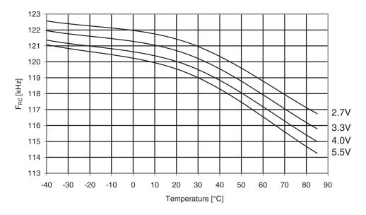
Figure 29-381. Atmel ATmega1284P: Watchdog oscillator frequency vs. temperature.
