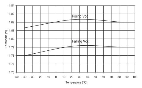
Figure 29-278. Atmel ATmega644PA: BOD threshold vs. temperature ( $V_{BOT} = 1.8V$ ).
