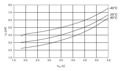
Figure 29-391. Atmel ATmega1284P: Watchdog timer current vs. V<sub>CC</sub>.
