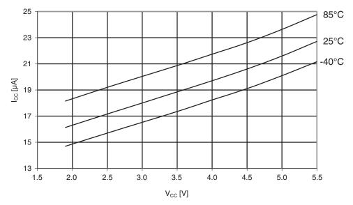
Figure 29-339.Atmel ATmega1284: Brownout detector current vs. V<sub>CC</sub>.
