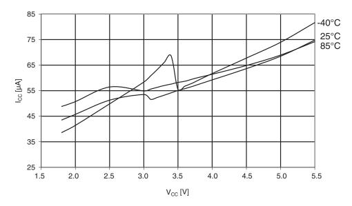
Figure 29-387. Atmel ATmega1284P: Analog comparator current vs. V<sub>CC</sub>.
