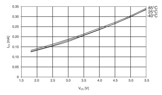
Figure 29-205. Atmel ATmega644A: Idle supply current vs. V<sub>CC</sub> (internal RC oscillator, 1MHz).
