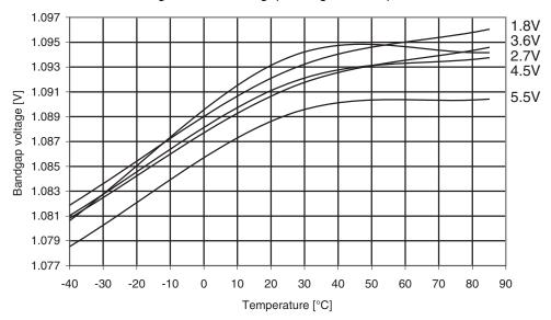
Figure 29-182. Atmel ATmega324PA: Bandgap voltage vs. temperature.
