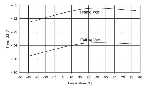
Figure 29-227. Atmel ATmega644A: BOD threshold vs. temperature (V<sub>BOT</sub> = 4.3V).
