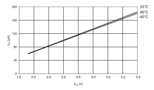
Figure 29-190.Atmel ATmega324PA: AREF external reference current vs. V<sub>CC</sub>.
