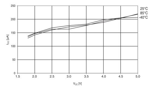
Figure 29-237. Atmel ATmega644A: ADC current vs.  $V_{CC}$  (AREF = AV<sub>CC</sub>).
