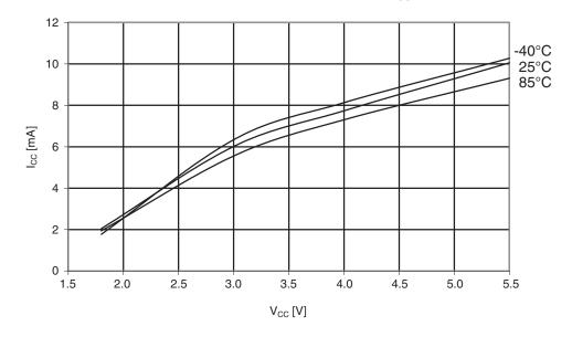
Figure 29-94. Atmel ATmega164PA: Programming current vs. V<sub>CC</sub>.
