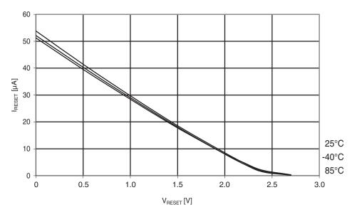
Figure 29-117. Atmel ATmega324A: Reset pull-up resistor current vs. reset pin voltage ( $V_{CC} = 2.7V$ ).
