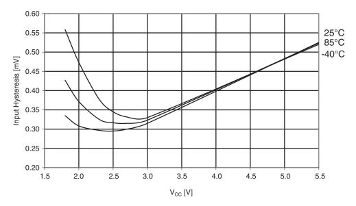
Figure 29-272. Atmel ATmega644PA: I/O pin input hysteresis vs. V<sub>CC</sub>.
