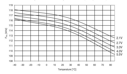
Figure 29-281. Atmel ATmega644PA: Watchdog oscillator frequency vs. temperature.
