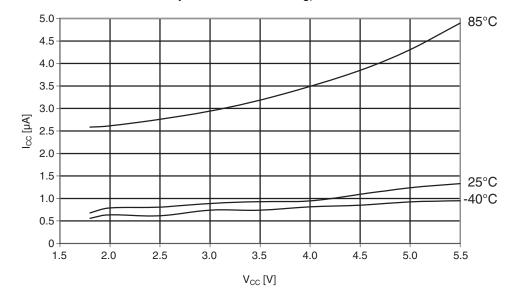
Figure 29-307.Atmel ATmega1284: Power-save supply current vs. V<sub>CC</sub> (watchdog timer disabled and 32kHz crystal oscillator running).
