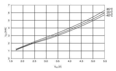
Figure 29-101. Atmel ATmega324A: Active supply current vs.  $V_{CC}$  (internal RC oscillator, 8MHz).
