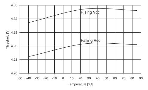
Figure 29-276. Atmel ATmega644PA: BOD threshold vs. temperature (V<sub>BOT</sub> = 4.3V).
