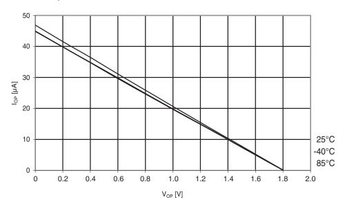
Figure 29-113.Atmel ATmega324A: I/O pin pull-up resistor current vs. input voltage ( $V_{CC} = 1.8V$ ).
