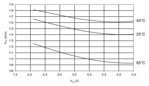
Figure 29-233. Atmel ATmega644A: Watchdog oscillator frequency vs. V<sub>CC</sub>.
