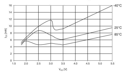
Figure 29-290.Atmel ATmega644PA: Programming current vs. V<sub>CC</sub>.
