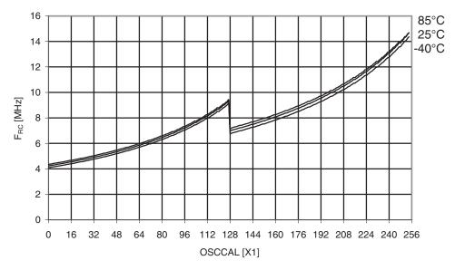
Figure 29-335. Atmel ATmega1284: Calibrated 8MHz RC oscillator vs. OSCCAL value.
