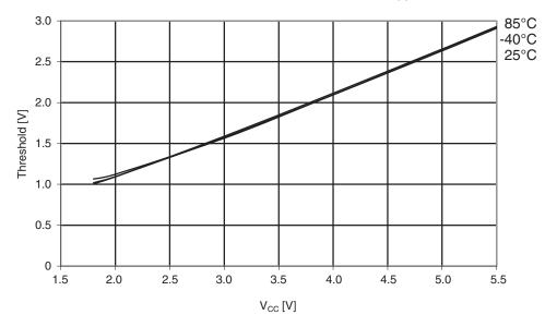
Figure 29-270. Atmel ATmega644PA: I/O pin input threshold vs.  $V_{CC}$  ( $V_{IH}$ , I/O pin read as '1').
