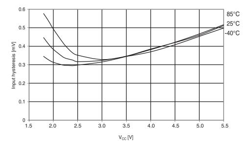
Figure 29-125. Atmel ATmega324A: I/O pin input hysteresis vs. V<sub>CC</sub>.
