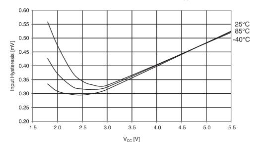
Figure 29-223. Atmel ATmega644A: I/O pin input hysteresis vs. V<sub>CC</sub>.
