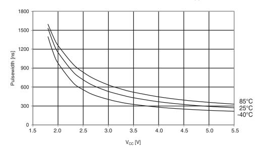
Figure 29-147. Atmel ATmega324A: Minimum reset pulsewidth vs. V<sub>CC</sub>.
