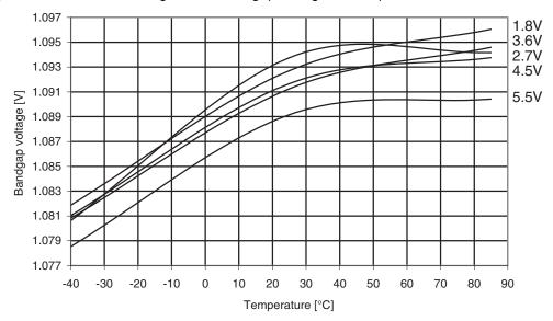
Figure 29-133. Atmel ATmega324A: Bandgap voltage vs. temperature.
