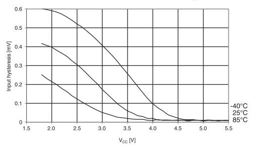
Figure 29-375. Atmel ATmega1284P: Reset pin input hysteresis vs. V<sub>CC</sub>.
