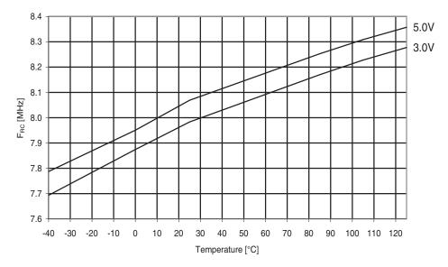
Figure 29-284. Atmel ATmega644PA: Calibrated 8MHz RC oscillator vs. temperature.
