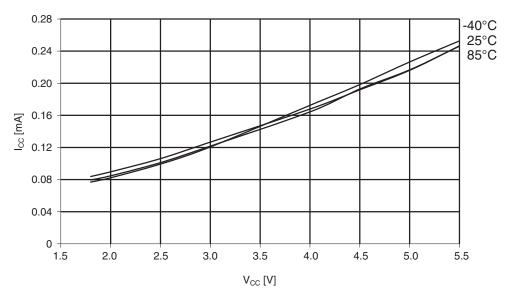
Figure 29-299. Atmel ATmega1284: Active supply current vs. V<sub>CC</sub> (internal RC oscillator, 128kHz).
