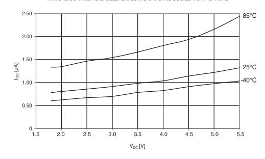
Figure 29-111.Atmel ATmega324A: Power-save supply current vs. V<sub>CC</sub> (watchdog timer disabled and 32kHz crystal oscillator running).
