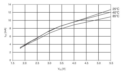
Figure 29-192. Atmel ATmega324PA: Programming current vs. V<sub>CC</sub>.
