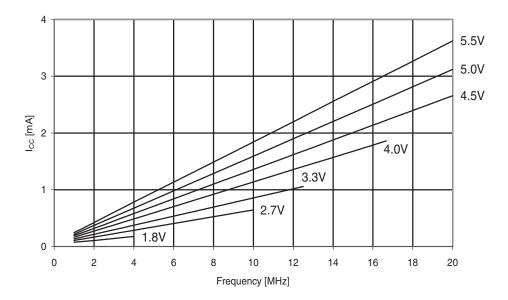
Figure 29-105. Atmel ATmega324A: Idle supply current vs. V<sub>CC</sub> (1 - 20MHz).
