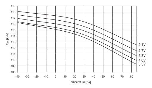
Figure 29-232. Atmel ATmega644A: Watchdog oscillator frequency vs. temperature.
