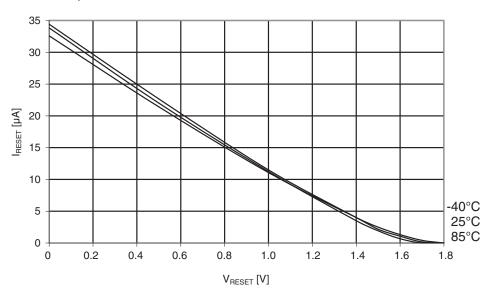
Figure 29-309. Atmel ATmega1284: I/O pin pull-up resistor current vs. input voltage ( $V_{CC} = 1.8V$ ).
