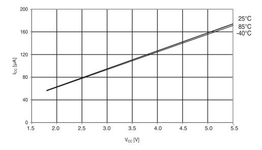
Figure 29-288.Atmel ATmega644PA: AREF external reference current vs. V<sub>CC</sub>.
