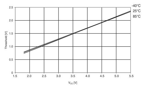
Figure 29-176. Atmel ATmega324PA: Reset pin input threshold vs.  $V_{CC}$  (V<sub>IL</sub>, I/O pin read as '0').
