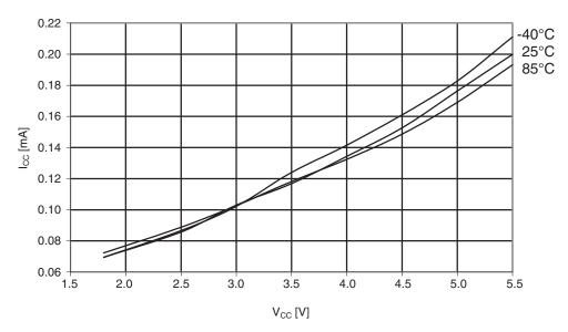
Figure 29-250.Atmel ATmega644PA: Active supply current vs. V<sub>CC</sub> (internal RC oscillator, 128kHz).
