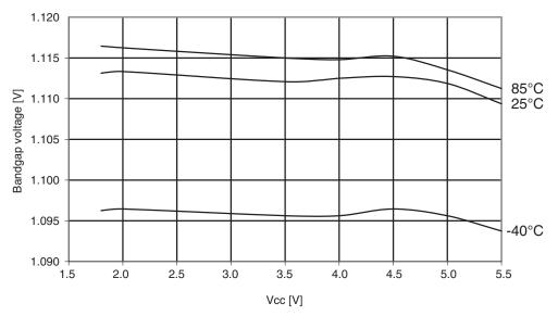
Figure 29-379. Atmel ATmega1284P: Calibrated bandgap voltage vs.  $V_{CC}$ .
