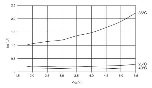
Figure 29-258.Atmel ATmega644PA: Power-save supply current vs. V<sub>CC</sub> (watchdog timer disabled and 32kHz crystal oscillator running).
