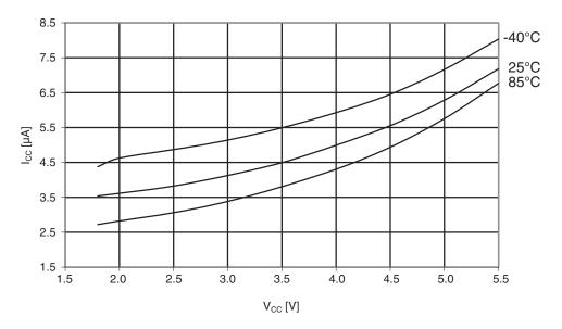
Figure 29-341. Atmel ATmega1284: Watchdog timer current vs. V<sub>CC</sub>.
