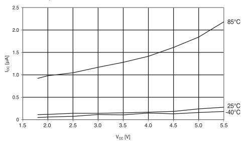
Figure 29-256.Atmel ATmega644PA: Power-down supply current vs. V<sub>CC</sub> (watchdog timer disabled).
