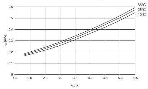
Figure 29-107. Atmel ATmega324A: Idle supply current vs. V<sub>CC</sub> (internal RC oscillator, 1MHz).
