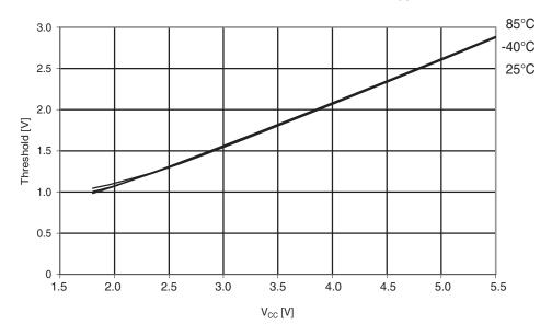
Figure 29-172. Atmel ATmega324PA: I/O pin input threshold vs.  $V_{CC}$  ( $V_{IH}$ , I/O pin read as '1').
