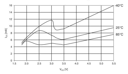
Figure 29-241.Atmel ATmega644A: Programming current vs. V<sub>CC</sub>.
