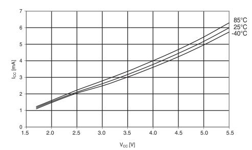
Figure 29-150. Atmel ATmega324PA: Active supply current vs.  $V_{CC}$  (internal RC oscillator, 8MHz).
