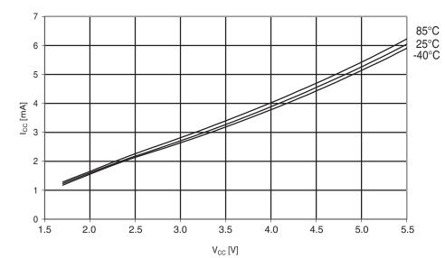
Figure 29-248.Atmel ATmega644PA: Active supply current vs. V<sub>CC</sub> (internal RC oscillator, 8MHz).
