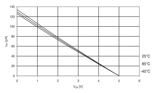
Figure 29-165. Atmel ATmega324PA: Reset pull-up resistor current vs. reset pin voltage ( $V_{CC} = 1.8V$ ).
