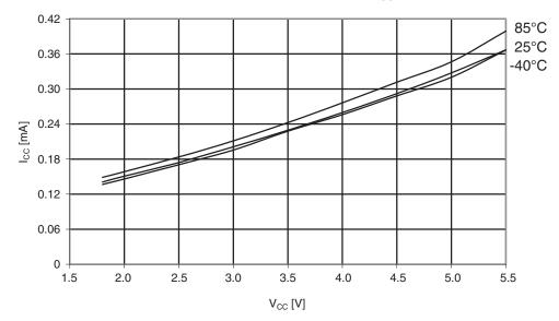
Figure 29-353. Atmel ATmega1284P: Idle supply current vs. V<sub>CC</sub> (internal RC oscillator, 1MHz).
