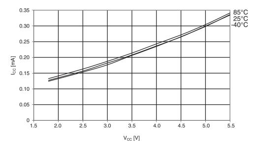
Figure 29-254. Atmel ATmega644PA: Idle supply current vs. V<sub>CC</sub> (internal RC oscillator, 1MHz).
