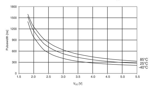
Figure 29-196. Atmel ATmega324PA: Minimum reset pulsewidth vs. V<sub>CC</sub>.
