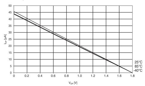
Figure 29-211.Atmel ATmega644A: I/O pin pull-up resistor current vs. input voltage ( $V_{CC} = 1.8V$ ).
