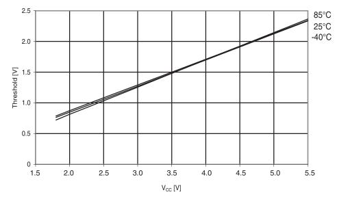
Figure 29-274.Atmel ATmega644PA: Reset pin input threshold vs. V<sub>CC</sub> (V<sub>IL</sub>, I/O pin read as '0').
