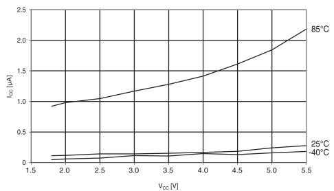
Figure 29-207.Atmel ATmega644A: Power-down supply current vs. V<sub>CC</sub> (watchdog timer disabled).
