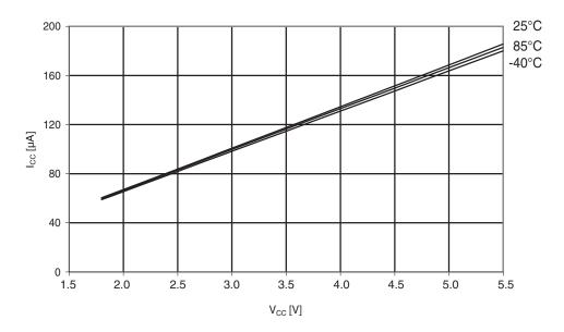
Figure 29-141.Atmel ATmega324A: AREF external reference current vs. V<sub>CC</sub>.
