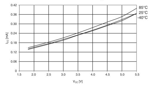
Figure 29-303. Atmel ATmega1284: Idle supply current vs. V<sub>CC</sub> (internal RC oscillator, 1MHz).
