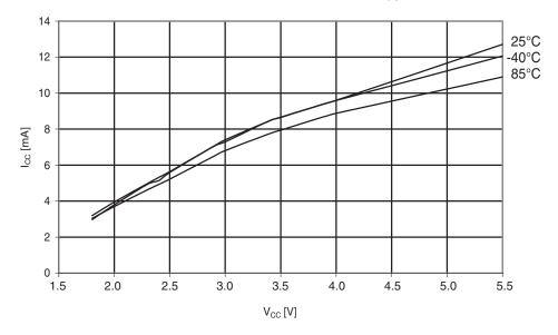
Figure 29-143. Atmel ATmega324A: Programming current vs. V<sub>CC</sub>.
