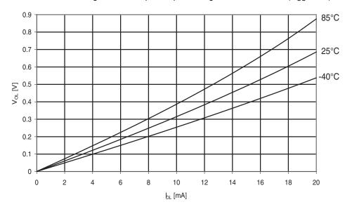
Figure 29-217. Atmel ATmega644A: I/O pin output voltage vs. sink current ( $V_{CC} = 3V$ ).
