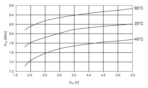
Figure 29-333. Atmel ATmega 1284: Calibrated 8MHz RC oscillator vs.  $V_{CC}$ .
