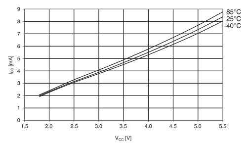
Figure 29-347. Atmel ATmega1284P: Active supply current vs.  $V_{CC}$  (internal RC oscillator, 8MHz).
