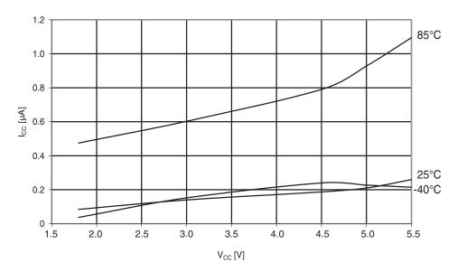
Figure 29-158.Atmel ATmega324PA: Power-down supply current vs. V<sub>CC</sub> (watchdog timer disabled).
