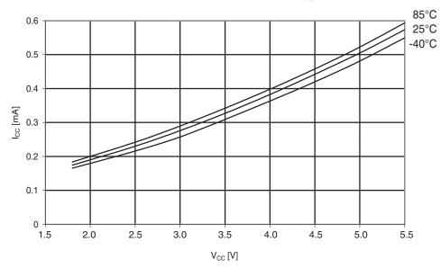
Figure 29-156. Atmel ATmega324PA: Idle supply current vs. V<sub>CC</sub> (internal RC oscillator, 1MHz).
