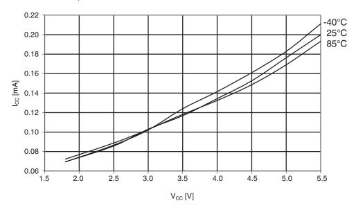
Figure 29-201. Atmel ATmega644A: Active supply current vs. V<sub>CC</sub> (internal RC oscillator, 128kHz).
