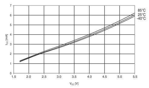
Figure 29-199. Atmel ATmega644A: Active supply current vs.  $V_{CC}$  (internal RC oscillator, 8MHz).
