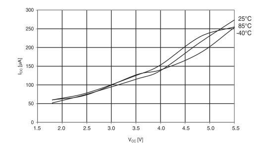
Figure 29-139. Atmel ATmega324A: ADC current vs.  $V_{CC}$  (AREF = AV<sub>CC</sub>).
