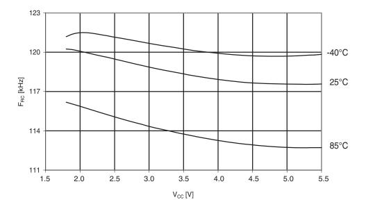
Figure 29-184.Atmel ATmega324PA: Watchdog oscillator frequency vs. V<sub>CC</sub>.
