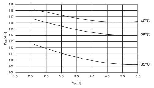
Figure 29-282. Atmel ATmega644PA: Watchdog oscillator orequency vs. V<sub>CC</sub>.
