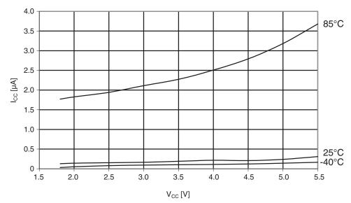
Figure 29-305.Atmel ATmega1284: Power-down supply current vs. V<sub>CC</sub> (watchdog timer disabled).
