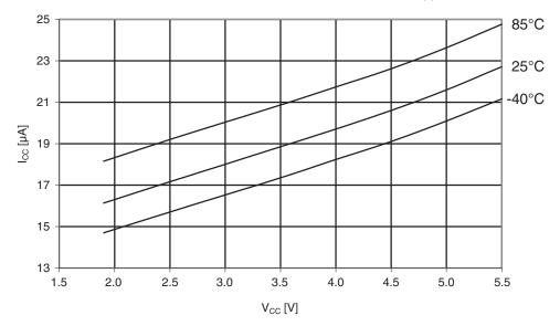
Figure 29-389. Atmel ATmega1284P: Brownout detector current vs. V<sub>CC</sub>.
