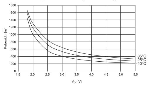
Figure 29-245. Atmel ATmega644A: Minimum reset pulsewidth vs. V<sub>CC</sub>.
