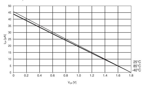
Figure 29-260. Atmel ATmega644PA: I/O pin pull-up resistor current vs. input voltage ( $V_{CC} = 1.8V$ ).
