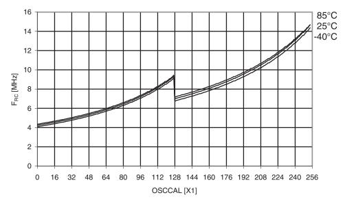
Figure 29-385. Atmel ATmega1284P: Calibrated 8MHz RC oscillator vs. OSCCAL value.
