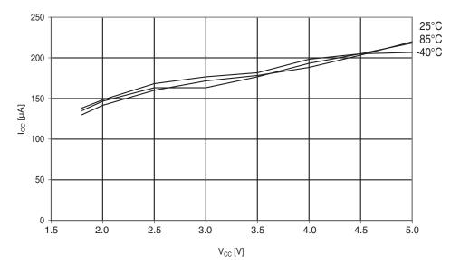
Figure 29-286. Atmel ATmega644PA: ADC current vs.  $V_{CC}$  (AREF = AV<sub>CC</sub>).
