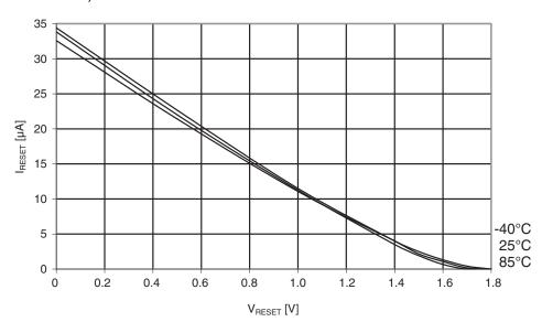
Figure 29-359. Atmel ATmega1284P: I/O pin pull-up resistor current vs. input voltage ( $V_{CC} = 1.8V$ ).
