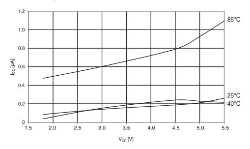
Figure 29-109.Atmel ATmega324A: Power-down supply current vs. V<sub>CC</sub> (watchdog timer disabled).
