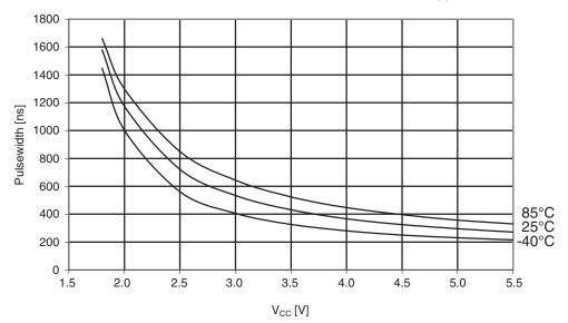
Figure 29-294. Atmel ATmega644PA: Minimum reset pulsewidth vs. V<sub>CC</sub>.
