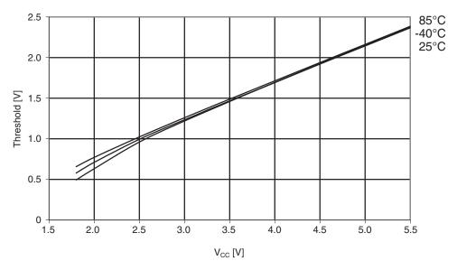
Figure 29-321.Atmel ATmega1284: I/O pin input threshold vs.  $V_{CC}$  (V<sub>IL</sub>, I/O pin read as '0').
