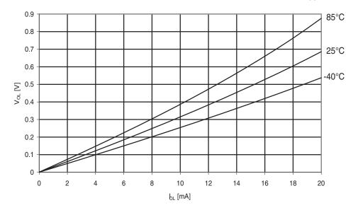
Figure 29-266.Atmel ATmega644PA: I/O pin output voltage vs. sink current (V<sub>CC</sub> = 3V).
