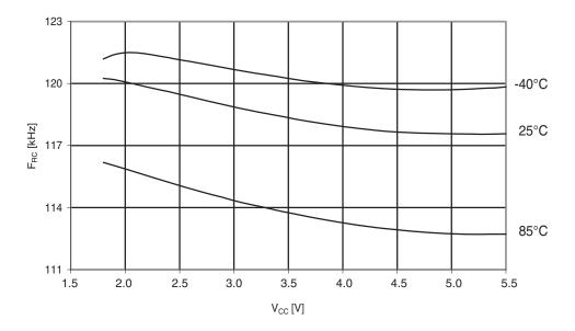
Figure 29-135.Atmel ATmega324A: Watchdog oscillator frequency vs. V<sub>CC</sub>.
