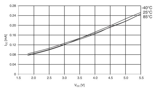
Figure 29-349.Atmel ATmega1284P: Active supply current vs. V<sub>CC</sub> (internal RC oscillator, 128kHz).
