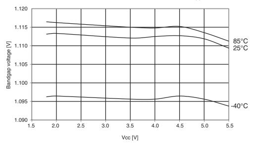
Figure 29-329. Atmel ATmega1284: Calibrated bandgap voltage vs. V<sub>CC</sub>.
