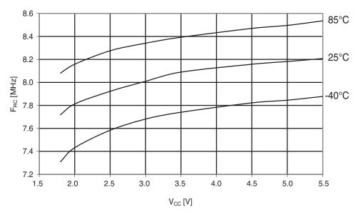
Figure 29-383. Atmel ATmega1284 P: Calibrated 8MHz RC oscillator vs.  $V_{CC}$ .
