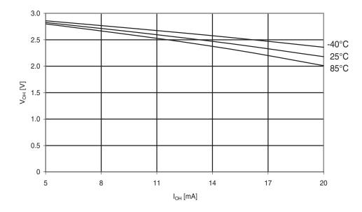
Figure 29-121. Atmel ATmega324A: I/O pin output voltage vs. source current (V<sub>CC</sub> = 3V).
