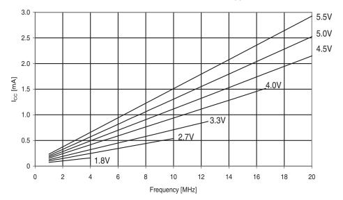
Figure 29-252. Atmel ATmega644PA: Idle supply current vs. V<sub>CC</sub> (1 - 20MHz).
