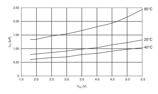
Figure 29-160.Atmel ATmega324PA: Power-save supply current vs. V<sub>CC</sub> (watchdog timer disabled and 32kHz crystal oscillator running).
