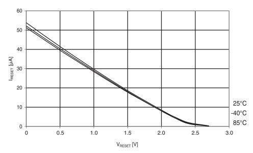
Figure 29-166. Atmel ATmega324PA: Reset pull-up resistor current vs. reset pin voltage  $(V_{CC} = 2.7V)$ .
