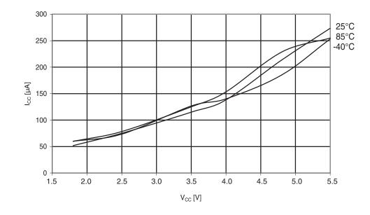
Figure 29-188. Atmel ATmega324PA: ADC current vs.  $V_{CC}$  (AREF = AV<sub>CC</sub>).
