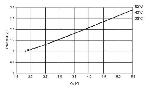
Figure 29-123. Atmel ATmega324A: I/O pin input threshold vs.  $V_{CC}$  ( $V_{IH}$ , I/O pin read as '1').
