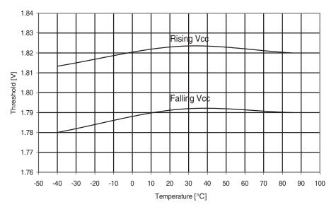
Figure 29-229. Atmel ATmega644A: BOD threshold vs. temperature ( $V_{BOT} = 1.8V$ ).
