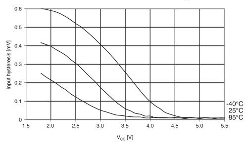
Figure 29-325. Atmel ATmega 1284: Reset pin input hysteresis vs. V<sub>CC</sub>.
