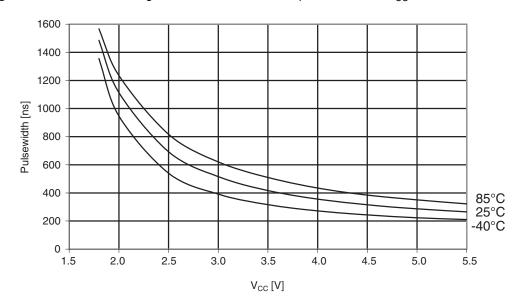
Figure 29-98. Atmel ATmega164PA: Minimum reset pulsewidth vs. V<sub>CC</sub>.
