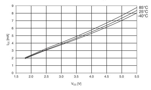
Figure 29-297. Atmel ATmega1284: Active supply current vs. V<sub>CC</sub> (internal RC oscillator, 8MHz).
