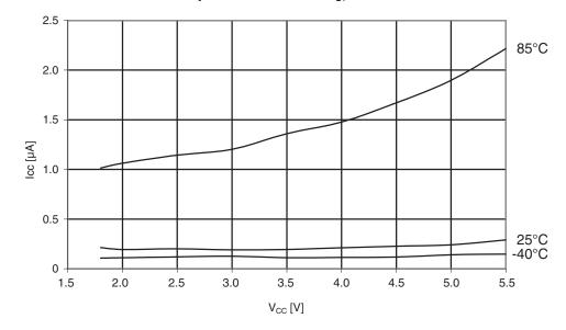
**Figure 29-209.**Atmel ATmega644A: Power-save supply current vs. V<sub>CC</sub> (watchdog timer disabled and 32kHz crystal oscillator running).
