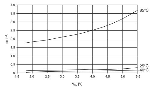
Figure 29-355.Atmel ATmega1284P: Power-down supply current vs. V<sub>CC</sub> (watchdog timer disabled).
