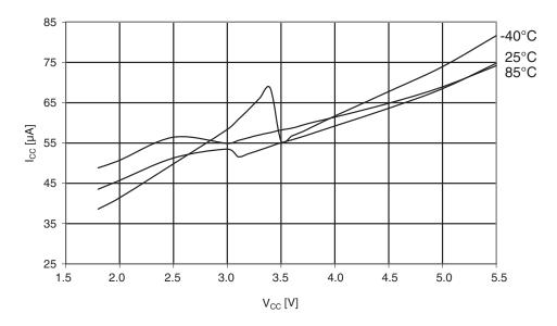
Figure 29-337. Atmel ATmega1284: Analog comparator current vs. V<sub>CC</sub>.
